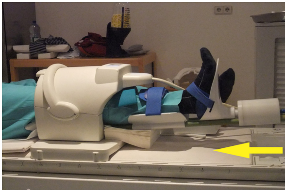
Fig. 1: MR compatible compression device is installed on the MR bed. Patient laying supine was fixed to the bed (fixation not shown on the figure). Knee coil was used for the signal acquisition. Yellow arrow shows the direction of pressure. Piston is located right on the figure. The compression device was controlled by the compressed air through the plastic tube, and the piston provided load to the foot plate.
