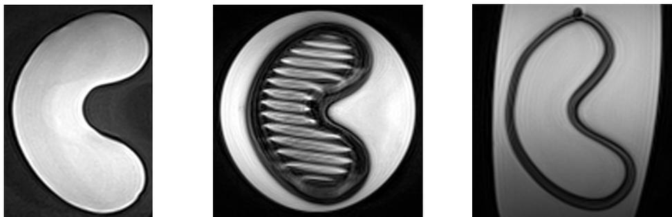
Fig. 3. Left: Image of the oil slick, GRE imaging sequence, TR = 800 ms, TE = 10 ms, slice thickness 2 mm. Center: Image of the soft magnetic sample, GRE, TR = 400 ms, TE = 10 ms, slice thickness 2 mm. Right: Image of the thin coil wire up into the oil slick shape, DC current 20 mA, GRE, TR = 500 ms, TE = 10 ms.
