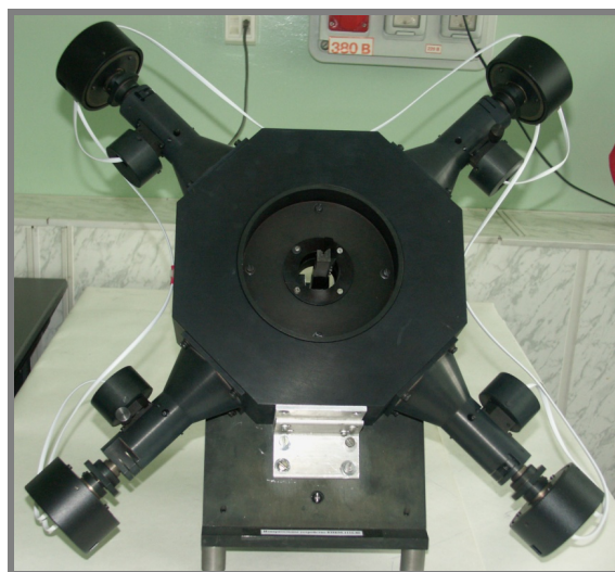
Fig. 2. Four-channel high-speed system for side surface inspection.
