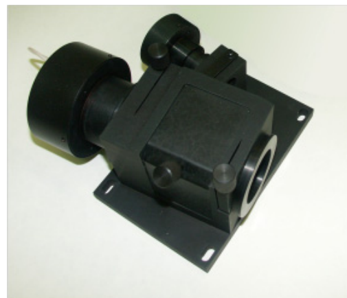
Fig. 5. Image recording unit for the edge surfaces inspection.
