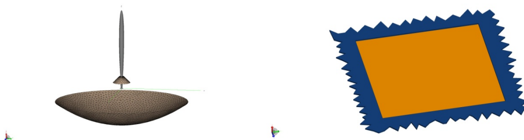
Fig. 4. a) Antenna of the level gauge and its radiation patterns, b) irregularly shaped absorber
