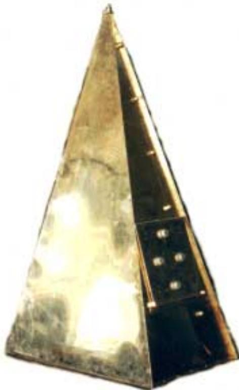
**Fig 8.** Photo of GTEM-cell
