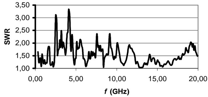
**Fig. 7.** SWR of GTEM-cell up to 20GHz
