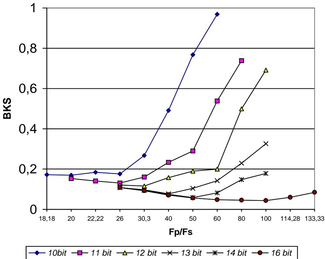
Fig.2 Correction quality index BKS in function of ratio  $F_p/F_s$  for various A/D converter word lengths .
