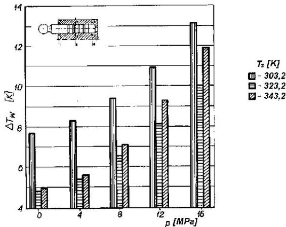
Fig. 3. Influence of temperature  $T_Z$  of oil supplied to the pump on temperature increase  $\Delta T_w$  of the kinematic pair piston-cylinder as a function of pressure  $p$
