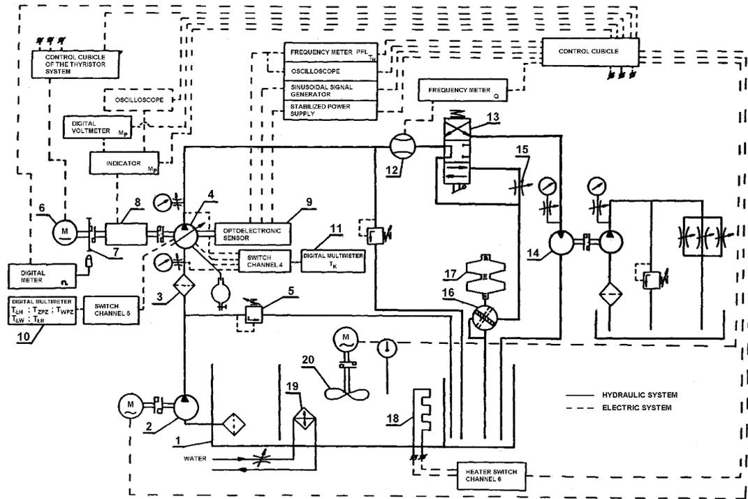
Fig. 1. Diagram of the hydraulic measuring stand
