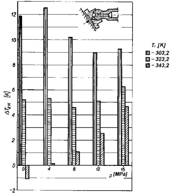
Fig.4. Influence of temperature  $T_Z$  of oil supplied to the pump on temperature increase  $\Delta T_{LH}$  of the kinematic pair slipper- swash plate as a function of pressure  $p$
