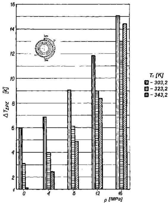
Fig. 5. Influence of temperature  $T_Z$  of oil supplied to the pump on temperature increase  $\Delta T_{ZPZ}$  of the kinematic pair cylinder block – valve plate as a function of pressure  $p$
