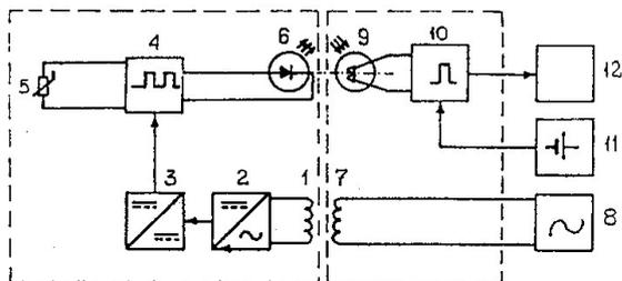
Fig. 2. Block diagram of the optoelectronic sensor for the measurements of cylinder block temperature
