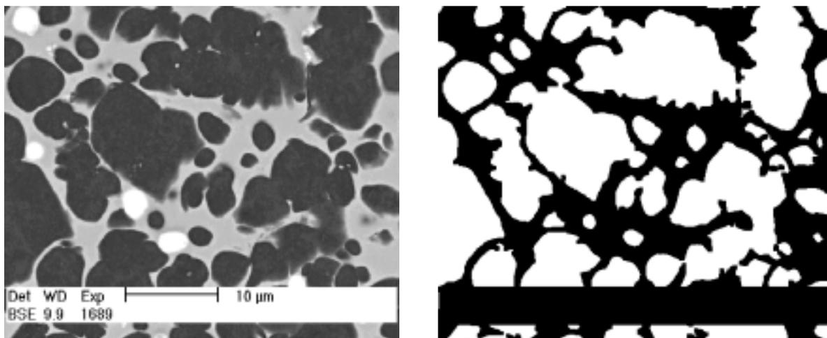
**Figure 4.** The sintering phase before (left), and after the image processing (right). White areas (right) are WNi grains. The holes disappeared after the processing.
