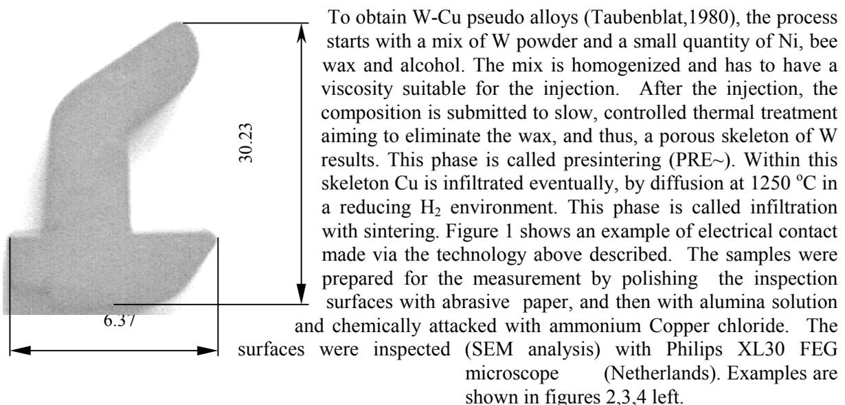
**Figure 1.** PIM made electrical contact
