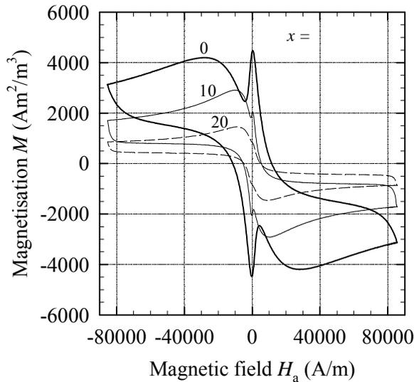
Figure 1. Effects of the silver doping levels on the magnetisation hysteresis loops  $M$  vs.  $H_a$  of the  $\text{YBa}_2\text{Cu}_3\text{O}_{7-\delta}/\text{Ag}$  sintered samples prepared from aqueous spray dried solutions of the corresponding nitrates, (series A).  $x$  denotes the doping level in wt % Ag.
