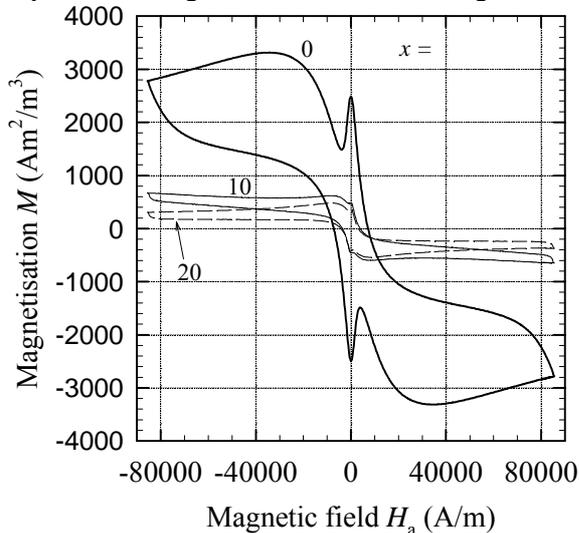
Figure 3. Effects of the silver doping levels on the magnetisation hysteresis loops  $M$  vs.  $H_a$  of the  $\text{YBa}_2\text{Cu}_3\text{O}_{7-\delta}/\text{Ag}$  sintered samples prepared by the citrate method, (series C).  $x$  denotes the doping level in wt % Ag.
