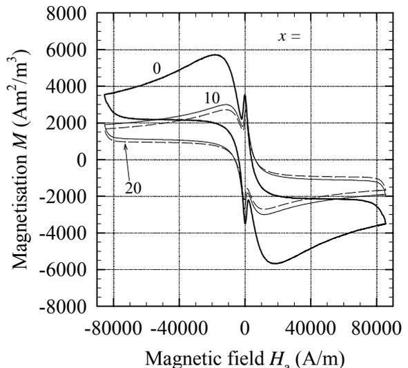
Figure 4. Effects of the silver doping levels on the magnetisation hysteresis loops  $M$  vs.  $H_a$  of the  $\text{YBa}_2\text{Cu}_3\text{O}_{7-\delta}/\text{Ag}$  sintered samples prepared by a direct solid state reaction of  $\text{Y}_2\text{O}_3$ ,  $\text{BaCO}_3$ ,  $\text{CuO}$  and  $\text{Ag}_2\text{O}$  powders, (series D).  $x$  denotes the doping level in wt % Ag.
