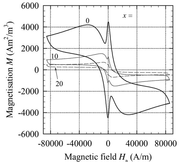
Figure 2. Effects of the silver doping levels on the magnetisation hysteresis loops  $M$  vs.  $H_a$  of the  $\text{YBa}_2\text{Cu}_3\text{O}_{7-\delta}/\text{Ag}$  sintered samples prepared from aqueous spray dried solutions of the corresponding nitrates including Ag, (series B).  $x$  denotes the doping level in wt % Ag.
