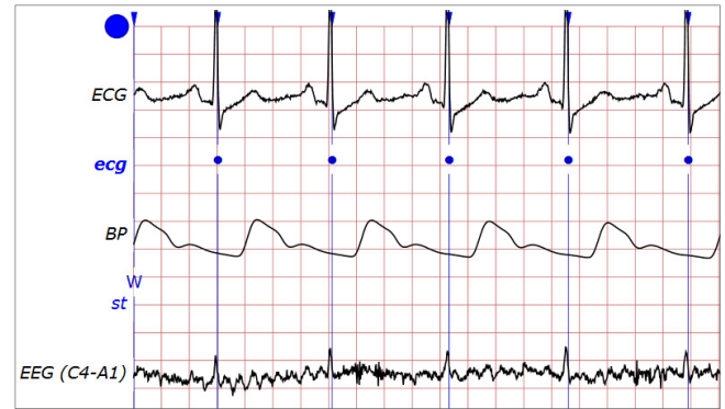
Fig.1. Annotated measurement from the MIT-BIH Polysomnographic database showing ECG, Blood Pressure and EEG signals. Note the pronounced ECG artefact contamination on the EEG channel (data record: https://physionet.org – slp/slp32 ).
